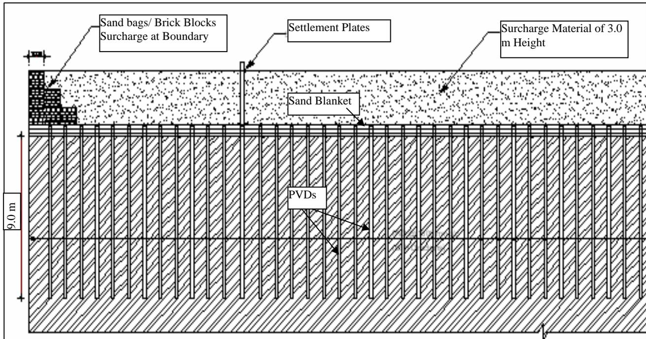
Figure 12. Detail of the ground improvement works (schematic).
