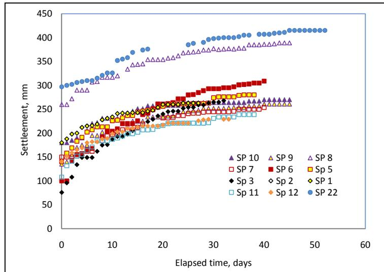
Figure 13. Ground settlements with time.
