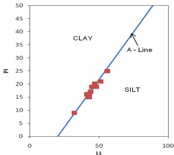
Figure 4. Data points with respect to A-line.
