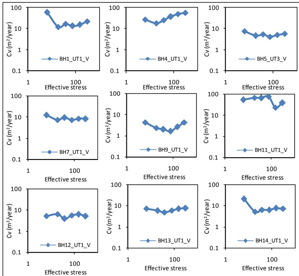
Figure 7. Coefficients of vertical consolidation against effective stresses.
