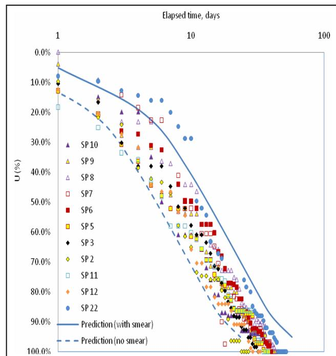
Figure 14. Measured and predicted Degree of Consolidation.
