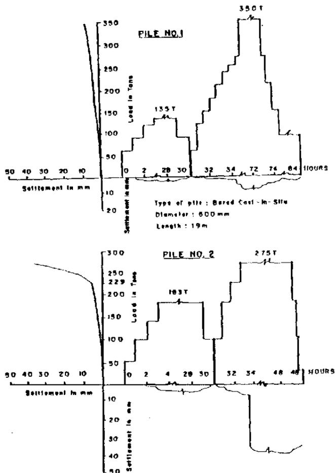
Figure 2: Static load test diagram.
