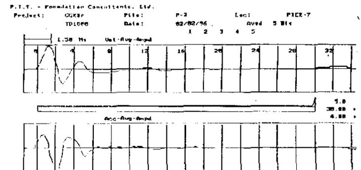
Figure 1: Defects (necking) in pile shaft formed at the tip of temporary casing.
