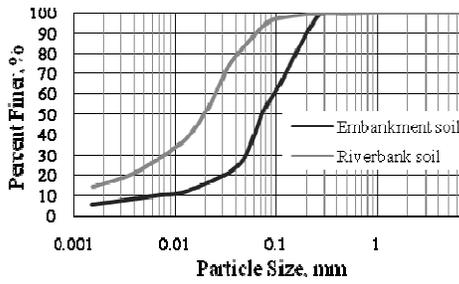
Fig. 2 Particle size distribution curves
