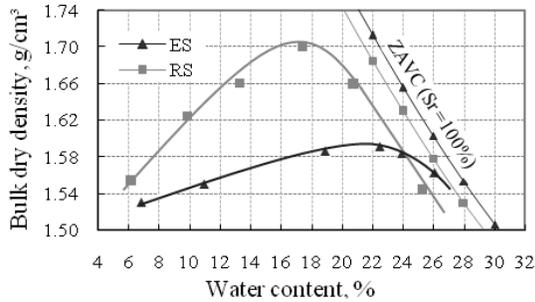
Fig. 3 Compaction curves of ES and RS
