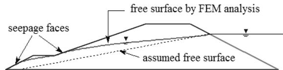
Fig. 9 Location of free surface and seepage faces
