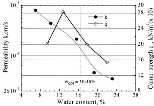
Fig. 6 Change of strength and permeability with water content of riverbank soil
