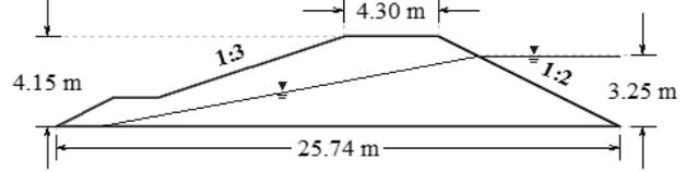
Fig. 8 Section of Manu river embankment
