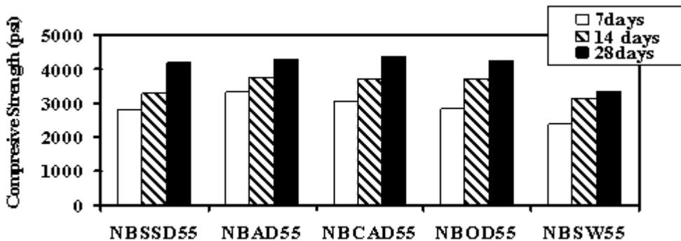
**Figure 5.3** Compressive strength of concrete made with aggregates with different moisture conditions.
