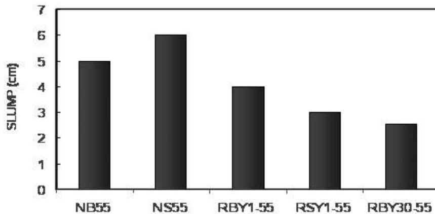
**Figure 6.1** Workability of concrete ( $w/cm = 0.55$ ).
