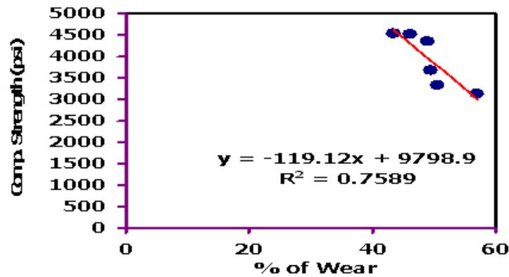
Figure 6.8 Compressive strength versus abrasion value.
