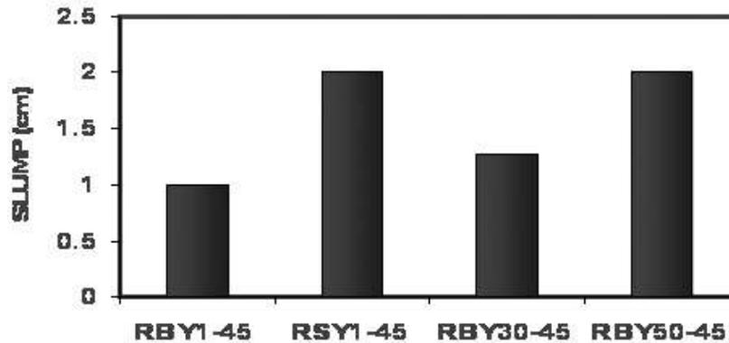
**Figure 6.2** Workability of concrete ( $w/cm = 0.45$ ).
