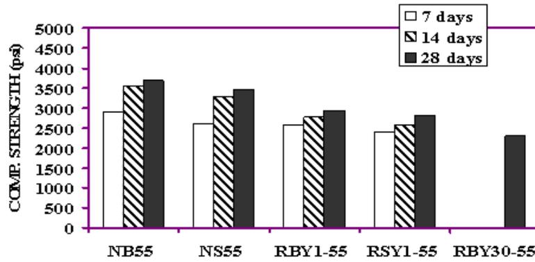
Figure 6.3 Compressive strength of concrete (w/cm =0.55).
