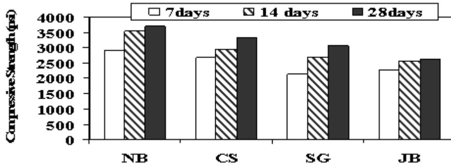
**Figure 5.2** Compressive strength of concrete made with different aggregates.
