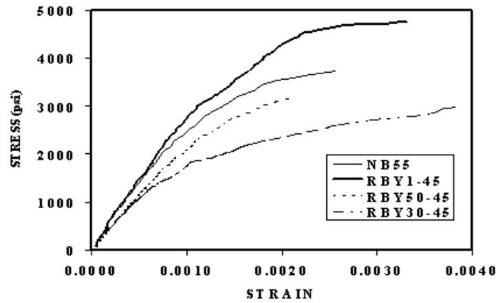
Figure 6.7 Stress-strain curves of concrete.
