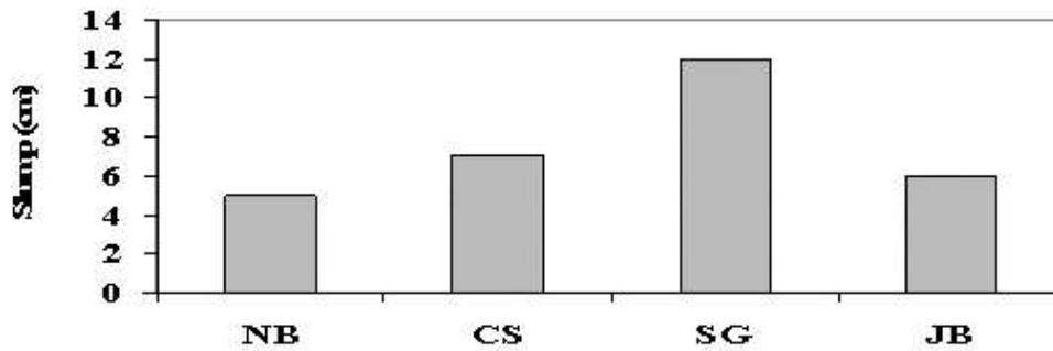
**Figure 5.1** Workability of concrete made with different aggregates (w/cm =0.55).
