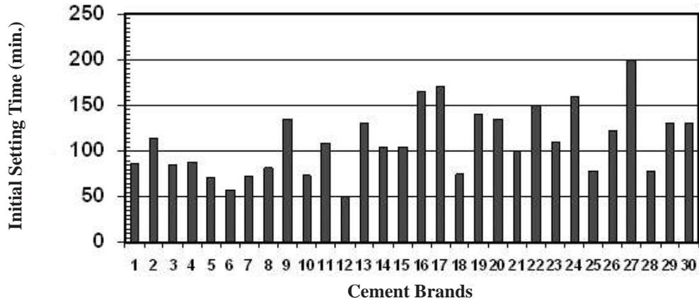
**Figure 4.1** Initial setting time of cement brands.
