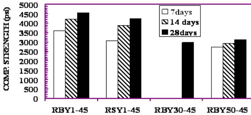
Figure 6.4 Compressive strength of concrete (w/cm =0.45).
